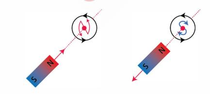
We can predict the direction induced current in different situation by using the Lenz's rule.
